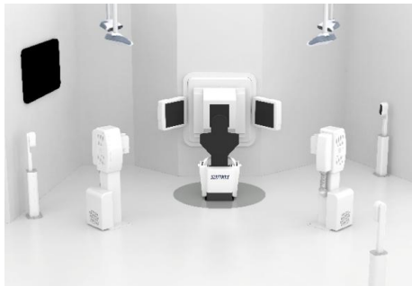
Figure 1: The MiniProton 360 treatment room contains alignment lasers, optical surface-monitoring cameras, and upright CBCT system to enable rapid and accurate patient positioning.
